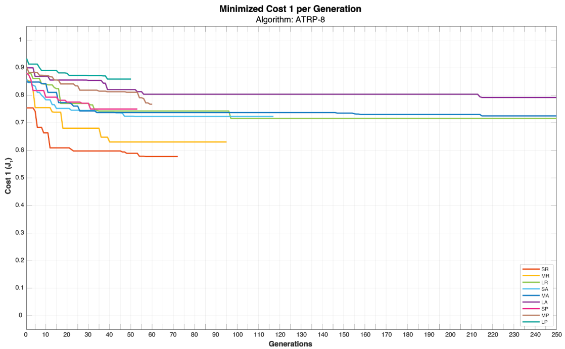
Figure 7.3 Cost 1 ( J ) optimised for Behavioural Algorithm ATRP-8, in 9 environments (SR, MR, LR, SA, MA, LA, SP, MP, and LP), with attractants and repellents.
