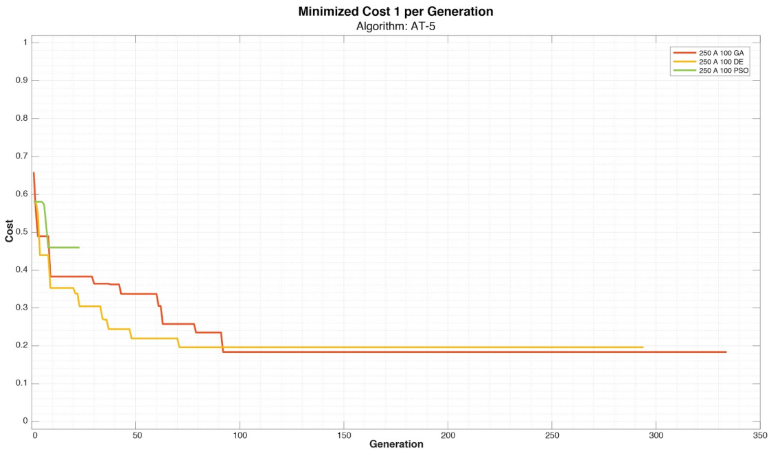
Figure 4.9 One instance of the experiments presented in Table 6.1: comparison of the minimisation of Cost 1 across Generations in 3 Evolutionary Algorithms (GA, DE, and PSO) using a Pool Size of 100 in the same environment (Field Size 250 with Average resource quality).
