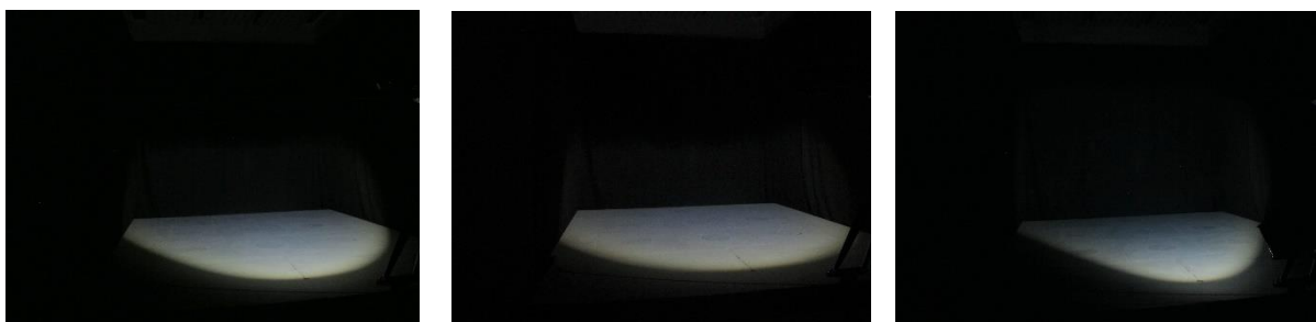
Figure 7. 10. Beam pattern on the floor surface ahead of the cyclists when the bicycle-mounted lamp was located at the helmet (left), handlebar (middle) and wheel hub (right).
