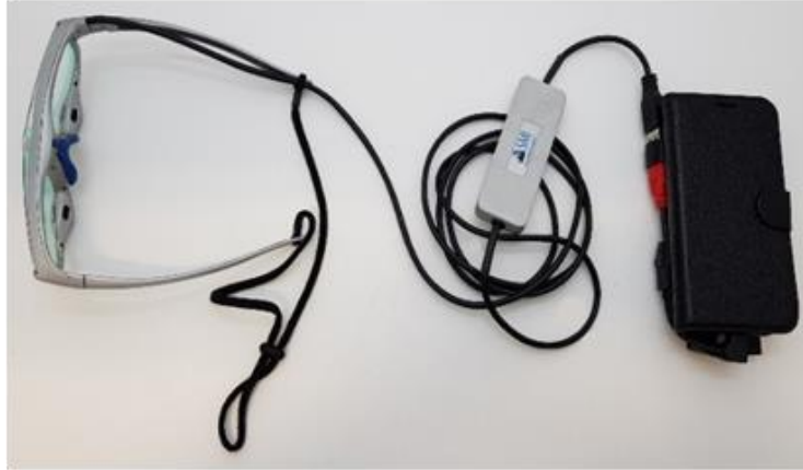
Figure 2. 2. SMI eye-tracking glasses and mobile recording device used in the studies reported in Chapters 4,5, and 6.
