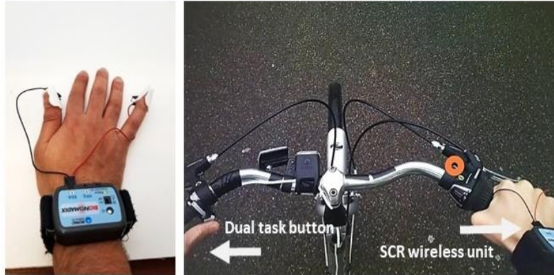
Figure 4.9. (Left) Electrodes for measuring SCR attached to the thumb and little finger of the right hand. (Right) Photograph of the bicycle handlebar to show the dual-task button and SCR wireless unit.
