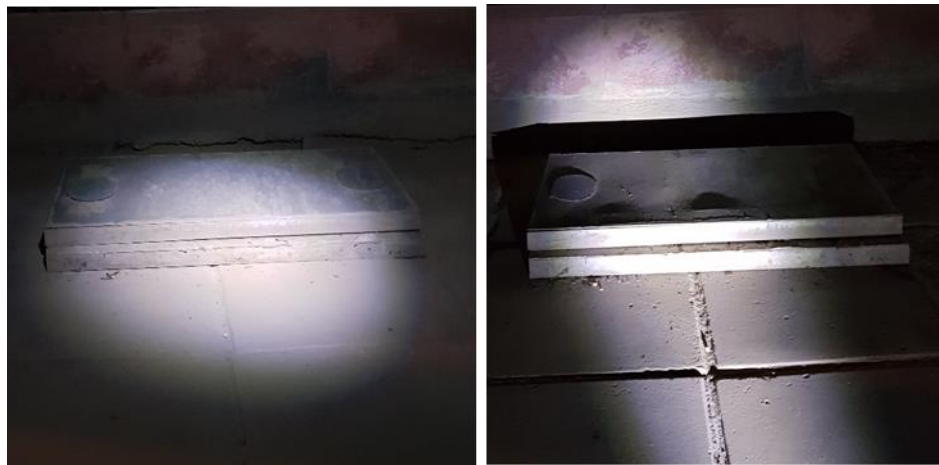
Figure 7. 7. The light projected from the helmet position (left) and from the hub (right) demonstrating how a change in bicycle light position influences the contrast between the side, top and surround of an object hence its conspicuity.
