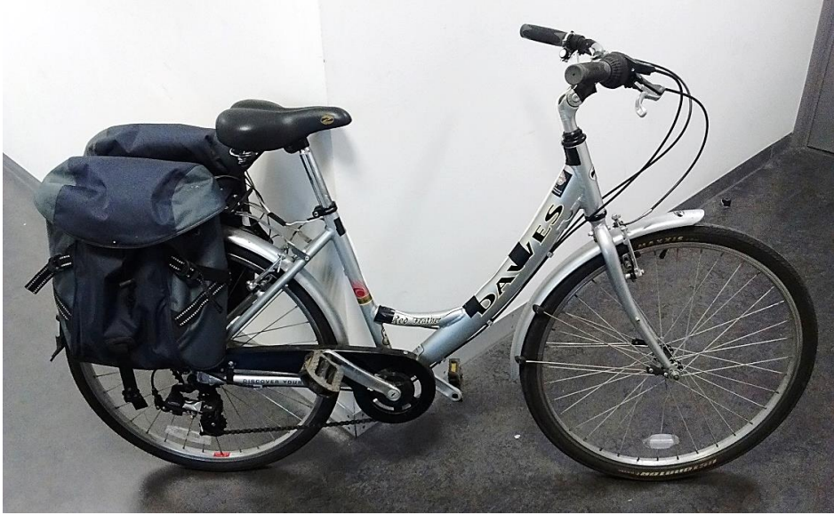
Figure 4.5. The bicycle used in the experiment. The rear panniers contain the EDA data acquisition unit (SCR), laptop, and external batteries.
