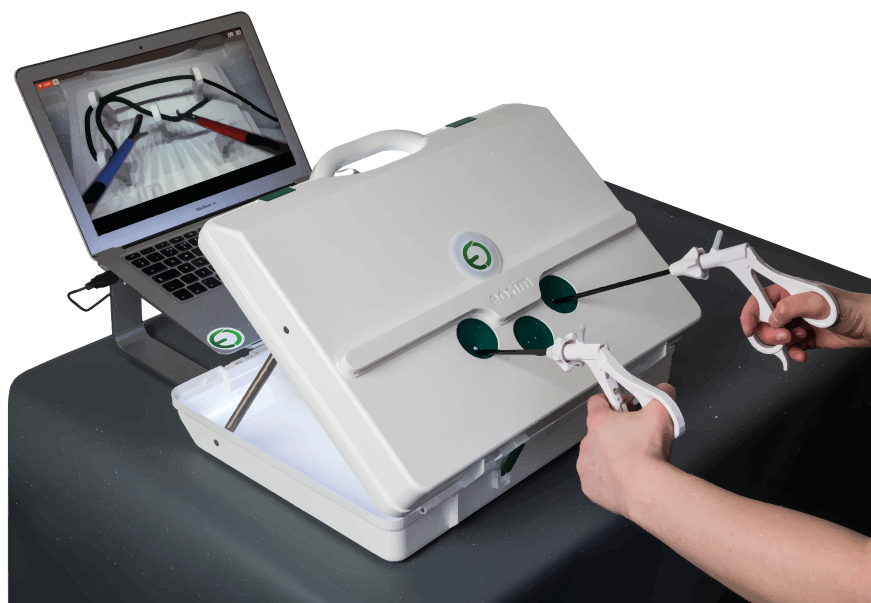
Figure 5-2 The set-up of the surgical simulator showing the performed surgical task which require passing the thread through the pegs.
