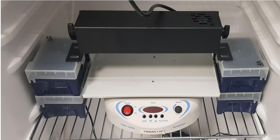
Figure S1: Photoirradiation setup – Consisting of the 400nm emitting LED backlight bar supported over a Grant-bio PMS-1000i microplate shaker.
