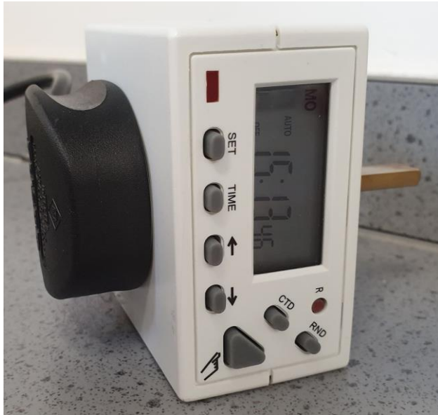
Figure S3: Photoirradiation control – The LED backlight bar was connected to the Timeguard Tg77 electrical timer plug allowing for up to 20 on/off cycles to be programmed.
