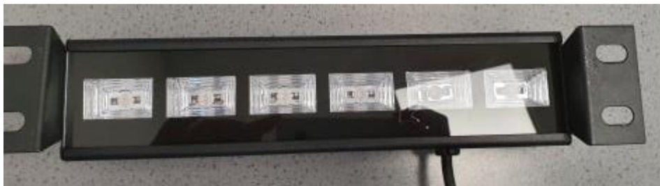
Figure S2: LED light bar – Consisting of 6x 3W LEDs housed in reflective units to provide a 120° angle of light.
