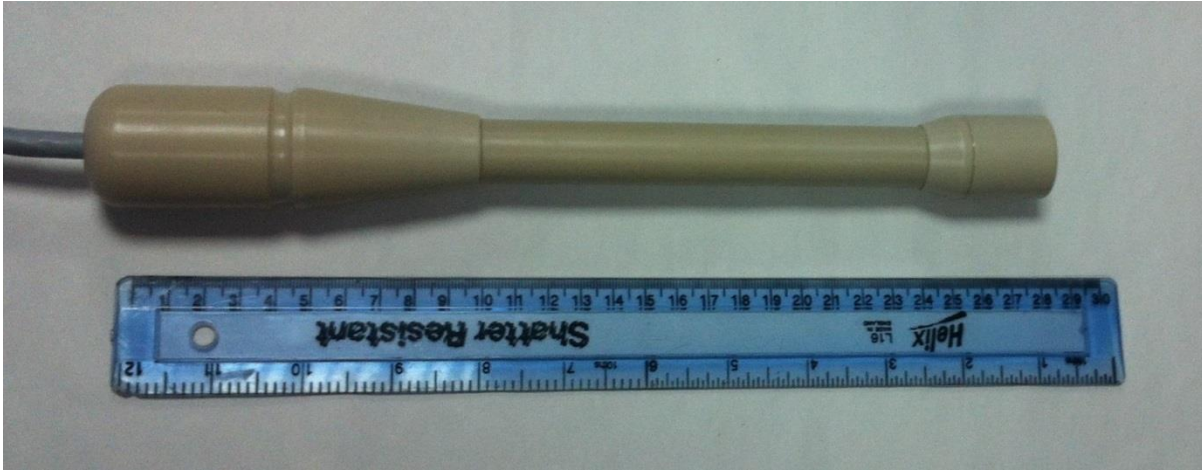
Figure 4.7. Mark II Magnetic induction spectrometry (MIS) probe. A ruler is shown for scale.
