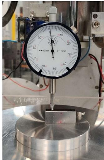
*Figure 4-9 – Shows the validation of the distance moved using a 5 mm slip block*
