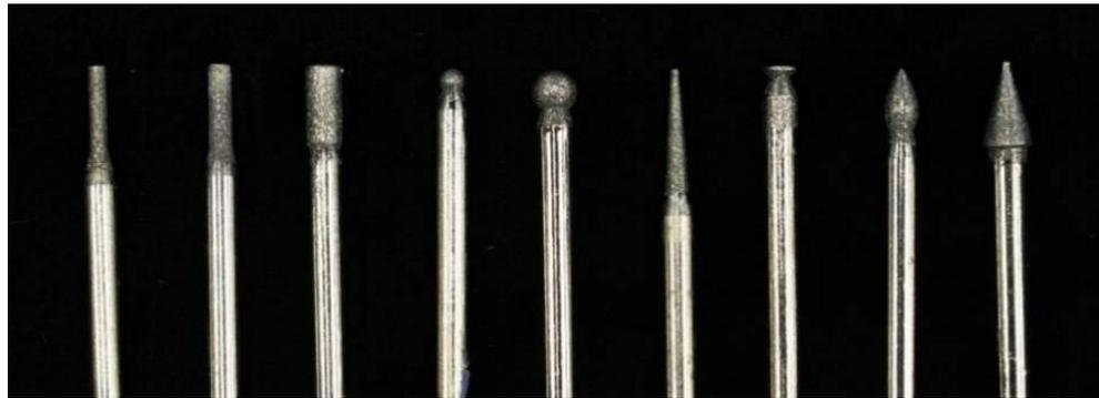
*Figure 3-24 – A range of PCD tooling with a range of cutter profiles*
