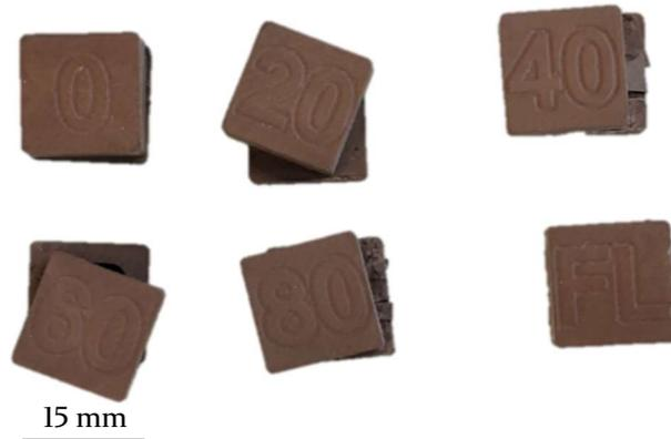
Figure 5-13 – shows the delaminated samples post sintering where samples 20, 40, 60 and 80 sintered in the orientations shown. Samples 0 and FL split into two separated pieces.
