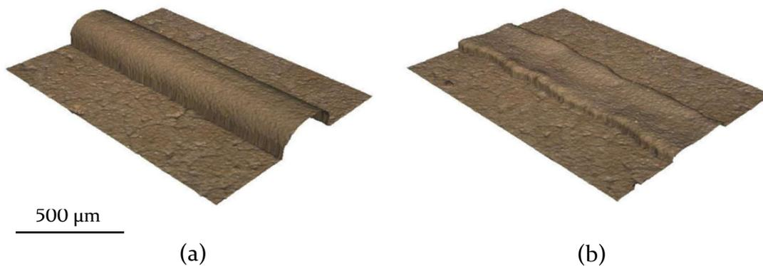
*Figure 5-1 – Shows the profiles generate for tracks produced with a 250  $\mu\text{m}$  straight-profile nozzle and constant printing height of 125  $\mu\text{m}$  on uncoated paper using a) Flowrate rate 40 $\mu\text{l}/\text{min}$ , Printing speed 650mm/min b) Flow rate 33 $\mu\text{l}/\text{min}$ , Printing speed 725mm/min w*
