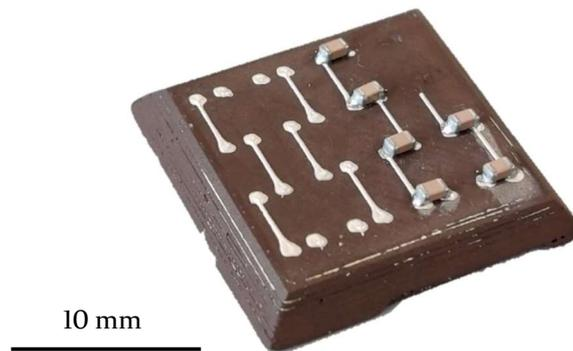
*Figure 6-8 – Shows an alumina substrate with sintered LTCC Ag tracks and 1210 components that have been reflowed with SAC solder at a peak temperature of  $249^{\circ}\text{C}$*
