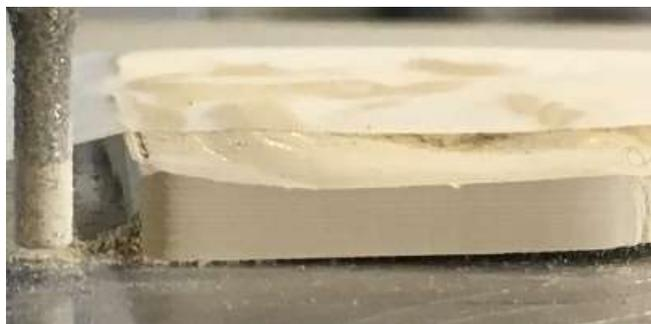
*Figure 3-26 – Shows the accumulation of machining debris on a PCD machining tool following a side milling operation*
