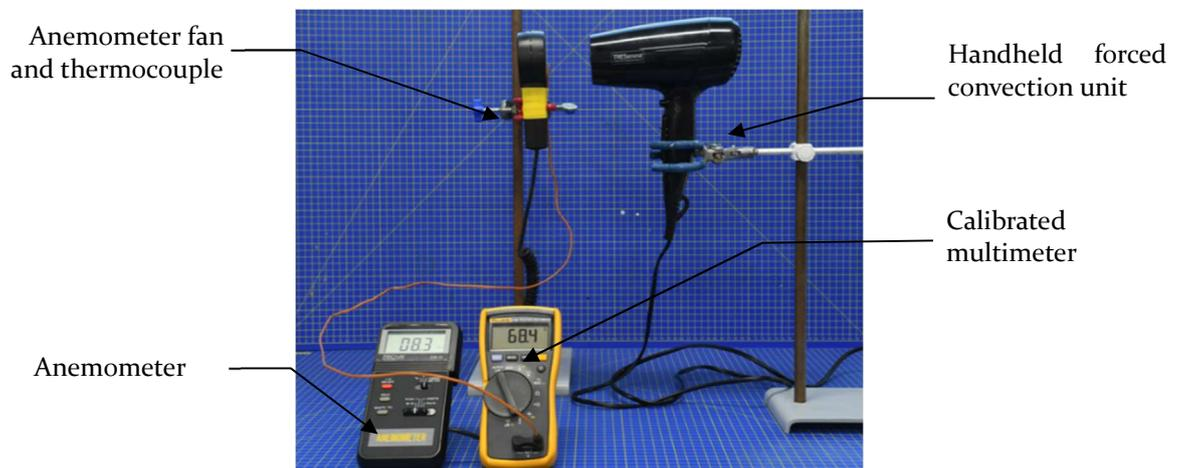
Figure 3-12 – Shows the configuration that was used to characterise the parameters of the handheld forced convection drying unit
