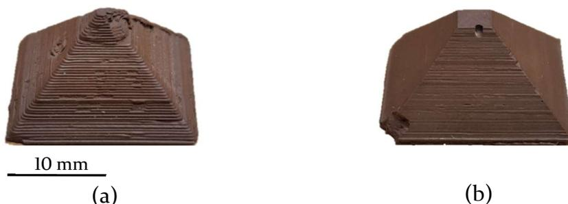
Figure 5-9 a) shows the sintered non-machined pyramid that exhibits a number of surface defects. b) shows the sintered machined pyramid
