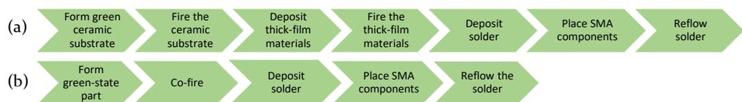
Figure 6-13 – a) shows the process of fabricating ceramic electronics when depositing thick-film materials onto sintered substrates b) shows the process of fabricating ceramic electronics using HTCC and LTCC materials
