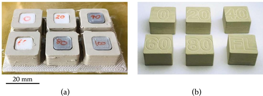
Figure 5-12 a) shows the placement of the prefabricated PLA support structures within the internal cavities. b) shows the enclosed geometries with the corresponding infill densities engraved on the top surface
