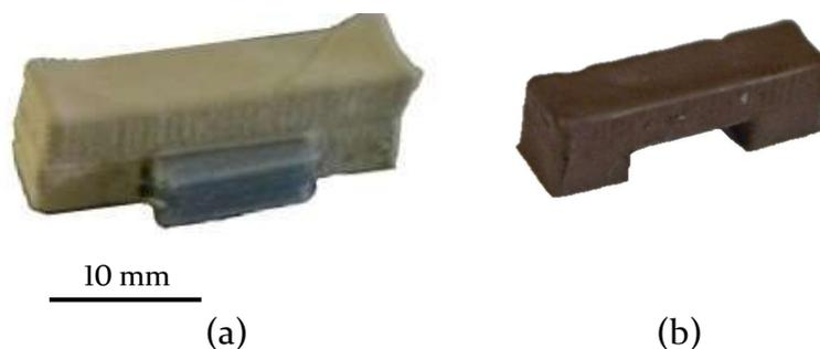
Figure 3-18 – (left) a spanning structure that was fabricated using a prefabricated PLA support structure. (right) shows the same sample post sintering.
