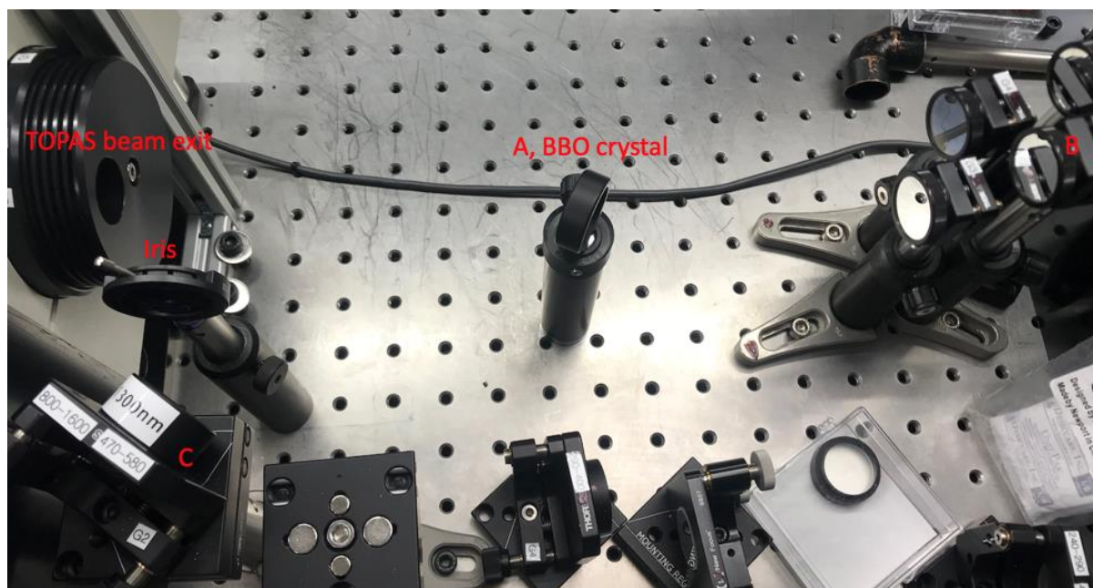
Figure 2.11 Photo shows the exit face of TOPAS. A is the BBO crystal used for frequency doubling of the gate, for alignment purposes. B is the first mirror for gate beam delivery to flups room. C is the second mirror for the delivery of the gate beam to the flups room. The iris is used for the adjustment of the first mirror, B .
