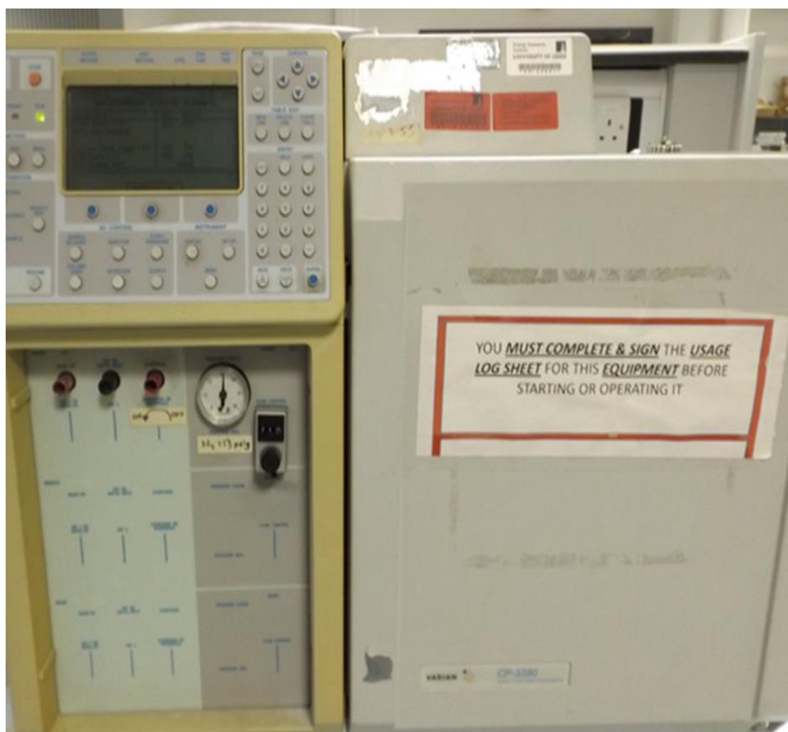
Figure 3.18. Gas chromatograph for gas analysis.
