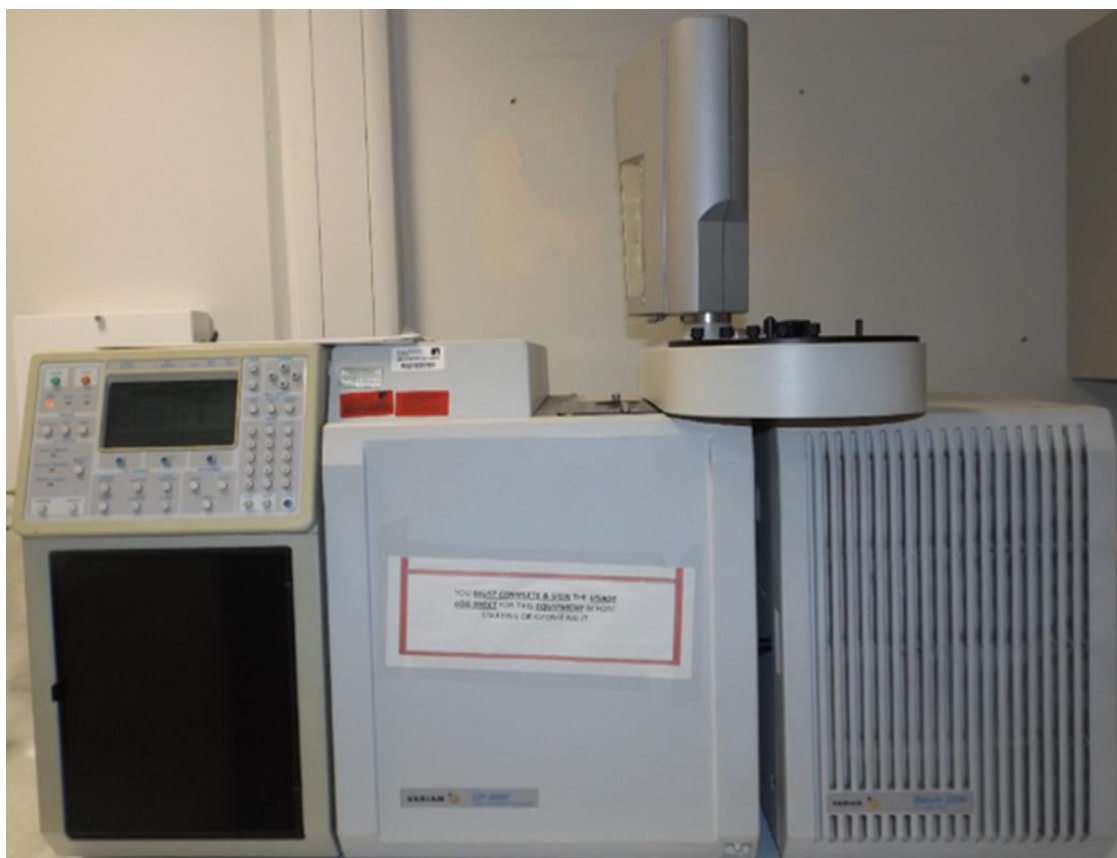
Figure 3.23. Gas chromatograph-mass spectrometer (GC-MS) for oil analysis.
