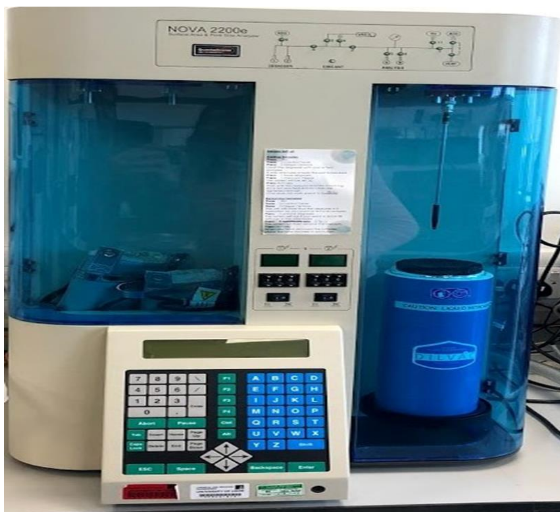
Figure 3.13. BET surface area and pore size NOVA 2200e instrument.
