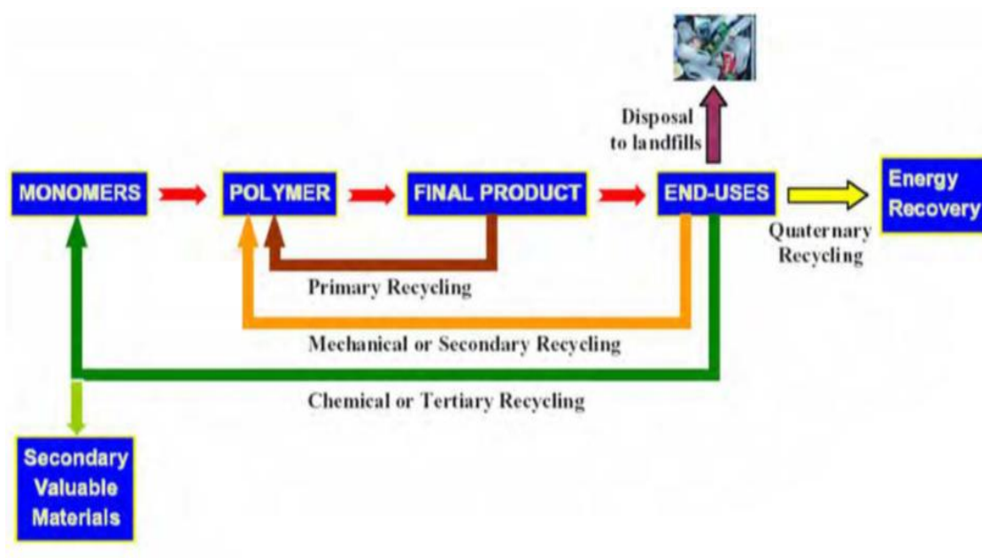
Figure 2.2. Illustration of polymer recycling techniques [6].
