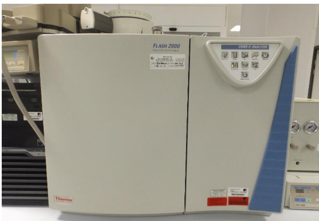
Figure 3.5. Illustration of the Elemental Analyser (CHNS-O).
