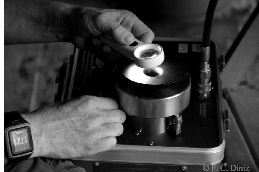
**Figure 2. 2** Equipment use to construt the vulnerability curves. **A:** Pneumatic apparatus to assess air discharge from the drying branch terminal end; **B:** Pressure chamber to assess leaf/xylem water potential.
