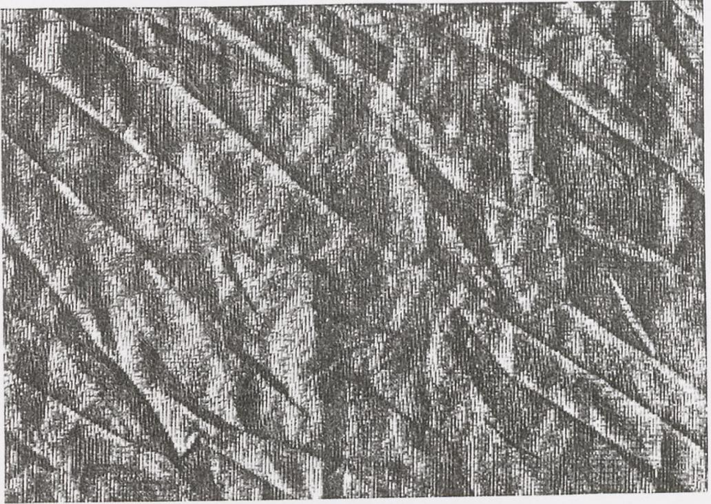
**Figure 5. 24** Scanned image of silk fabric treated with 6% w/w BTCA, a 1:1 molar ratio of SHP and 1% w/w Ceranine L (Clariant) that has been washed using a standard detergent on a delicate wash cycle and line dried.
