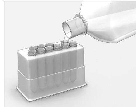
Figure 10: Filling the Pre-wash cassette
