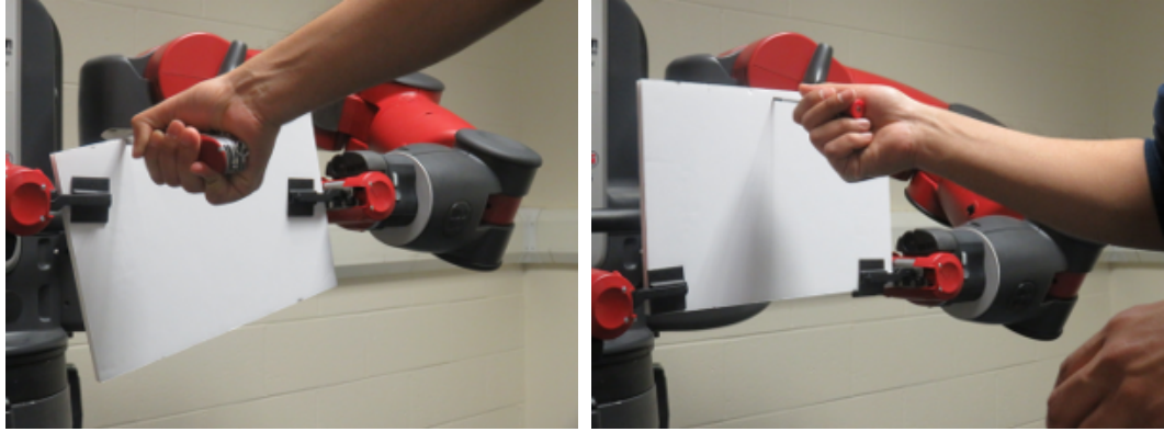
(a) The object slides between fingers due to insufficient frictional forces.
