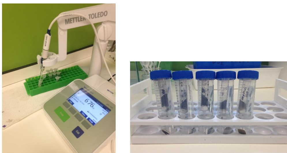
Figure 5. 1. Pore water pH analysis (left figure) and Falcon tubes containing the syringes with 3g of the sediment ready for the extraction of the pore water (right figure).
