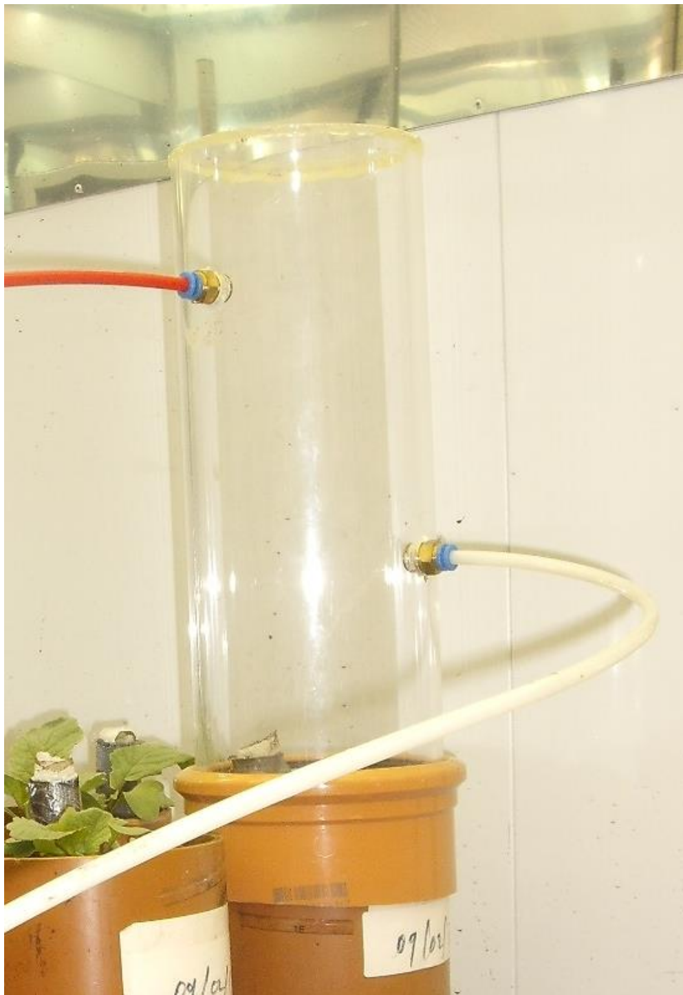
Figure 3.3: The transparent headspace chamber for gas flux used for the CO 2 and CH 4 concentration measurements from plants and soil under controlled lighting conditions (e.g. Net Ecosystem Exchange).
