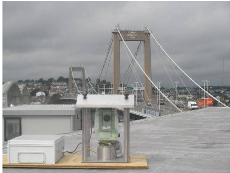
Figure 3.4: Robotic Total Station installed on the roof of the Tamar Bridge office
