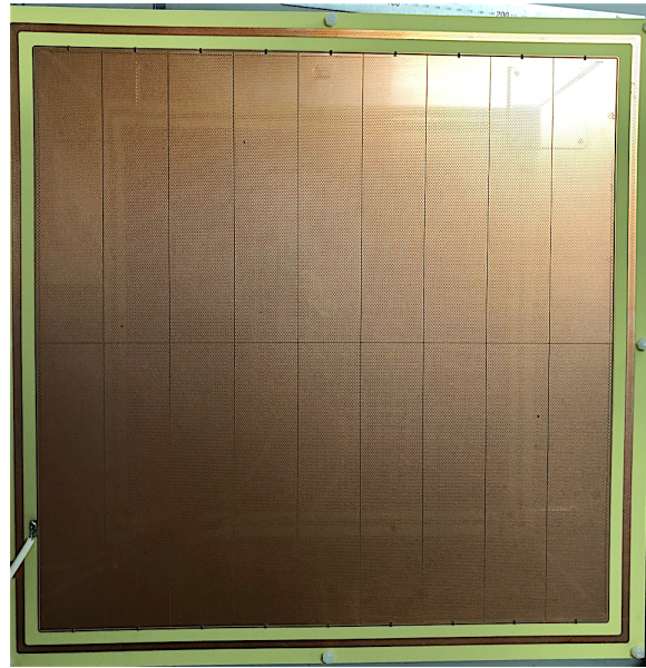
Figure 8.1: Large area ThGEM produced at CERN. The segmented side is shown with the surrounding veto ring. The surface mounted resistors can be seen connected to the segmented pads.
