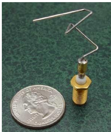
Fig. 2.5 An evolved antenna based on a specific NASA aerospace application. The image reprinted from Hornby et al. (2006).
