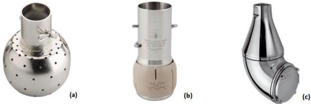
**Fig. 2. 32:** Exemplar CIP nozzles: (a) static spray ball (b) rotary spray head (c) rotary jet head (Sørensen, Accessed: 7/1/19).
