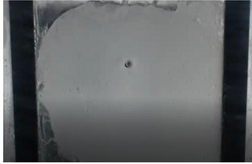
**Fig. 4. 9:** 300 s cleaning,  $1 \text{ lmin}^{-1}$  jet, 1.9 mm WSP thickness, water temperature  $20^\circ\text{C}$ .
