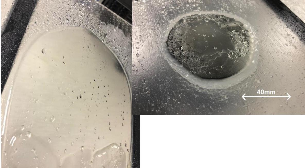
**Fig. 5. 31:** Left: long-time (300 s) clean area close-up ( $2.5 \text{ lmin}^{-1}$  spray, 0.19 mm WSP thickness, water temperature  $40 \text{ }^{\circ}\text{C}$ ), Right: long-time cleaned area close-up ( $2.5 \text{ lmin}^{-1}$  spray, 0.19 mm WSP thickness, water temperature  $20^{\circ}\text{C}$ ).
