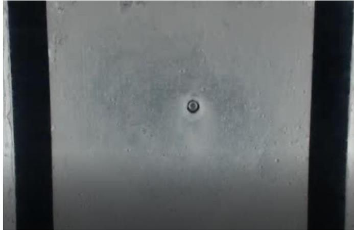
**Fig. 4. 6:** 300 s cleaning,  $1 \text{ lmin}^{-1}$  jet, 0.95 mm WSP thickness, water temperature  $20 \text{ }^{\circ}\text{C}$ .
