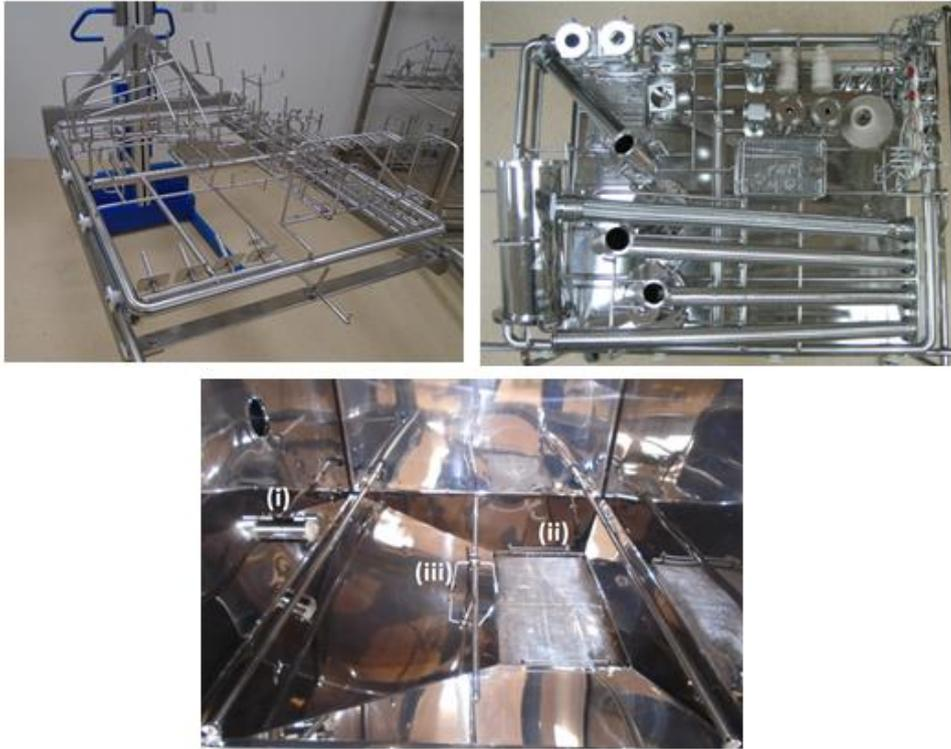
**Fig. 2. 34:** **a)** Wash rack unloaded. Each pipe section can be seen leading to a nozzle on to which a component is loaded **(b)** Wash rack with disassembled components loaded on to jet/spray nozzles **(c)** Wash rack is loaded into washer via coupling (i), water is recirculated via sump (ii) rinse of the chamber is performed by rotating jet arm (iii) (Rodgers et al., 2019).
