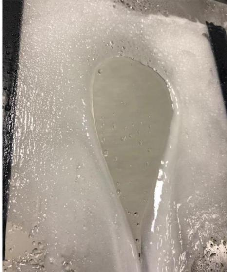
**Fig. 5. 36:** Long-time (300 s) clean area close up (1 lmin<sup>-1</sup> spray, 0.95 mm WSP thickness, water temperature 40 °C).
