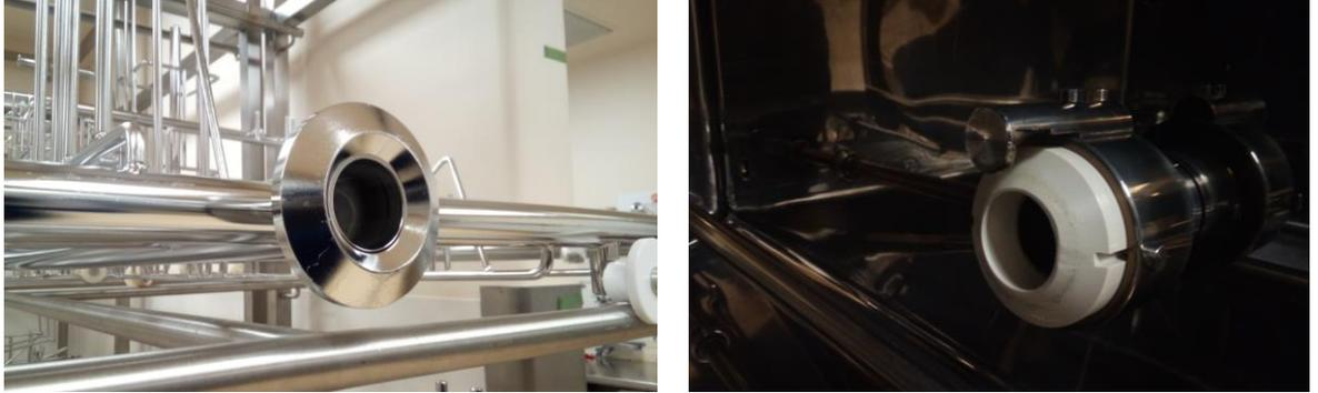
**Fig. 3. 1:** Coupling mechanism: Left: Female fitting on rack, right: male fitting in washer.
