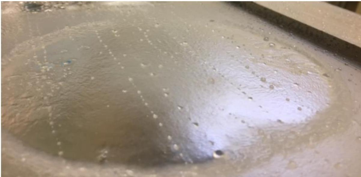
**Fig. 5. 29:** Cleaned area close-up after one hour of cleaning:  $2.5 \text{ lmin}^{-1}$  spray, 0.19 mm WSP thickness, water temperature  $20^\circ\text{C}$ , 125 mm standoff.
