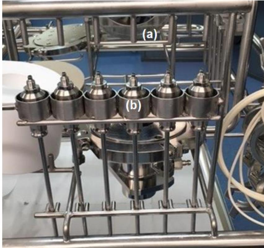
**Fig. 3. 19:** Rack 2 position of filling needles (b) cleaned by vertically aligned impinging jets (a).
