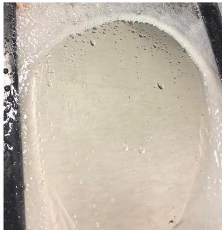
**Fig. 5. 33:** Long-time (300 s) clean area close up (2.5 lmin<sup>-1</sup> spray, 0.19 mm WSP thickness, water temperature 60 °C).
