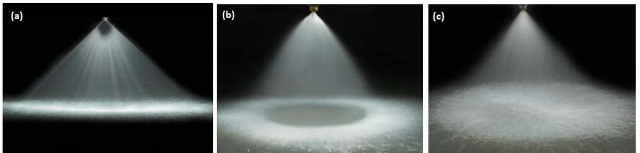
Fig. 2. 7: Spray distributions: a) Flat fan, b) Hollow cone, c) Full cone (PNR, Accessed: 27/2/19).
