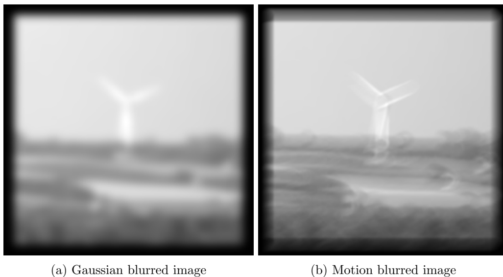
Figure 2.5: Exact image from Figure 2.4 blurred with Gaussian and motion PSFs shown in Figure 2.3
