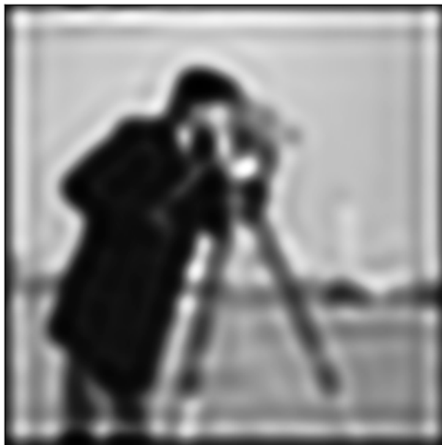
Figure 2.8: Image showing ringing artifacts in an image deconvolved by Lucy Richardson deconvolution
