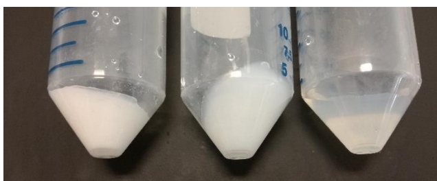
Figure 5-12: BIS synthesised at pH 7 using PAH as additive, before removing the additive through acid elution. From left to right: BIS at pH 7, BIS at pH 5 and BIS at pH 2.
