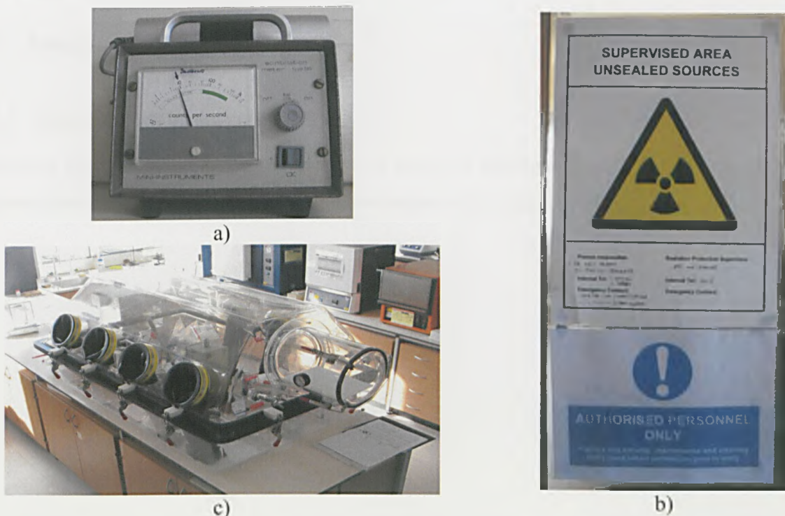
Figure 3.3: Safety equipment, a) Geiger counter; b) sign placed on laboratory door; and c) Glove box used for radioactive materials.
