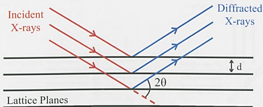
Figure 3.12: Diffraction of X-rays within a crystal.
