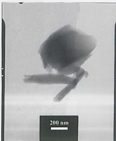
Figure 7.36: Picture showing amorphous sample on edge of carbon film, picture is taken before beam damage was apparent.
