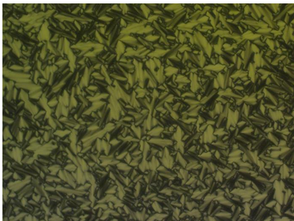
Figure 2-19: Photomicrograph of Pt-3 , taken at 165 °C upon cooling from the isotropic liquid.
