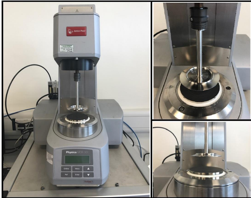
Figure 3.2 The Rheometer for the measurement of rheology
