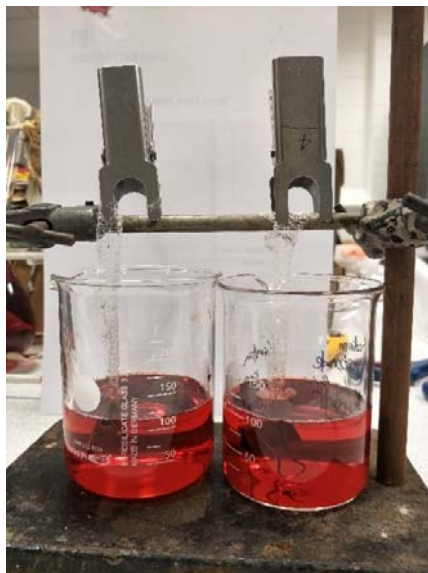
Figure 3.22 Vertical wicking test using wicking solution.
