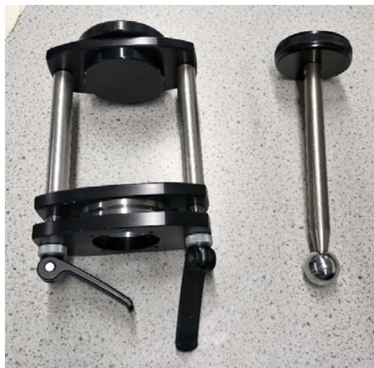
Figure 3.24 Ball burst tooling clamp (left) and ball probe (right).
