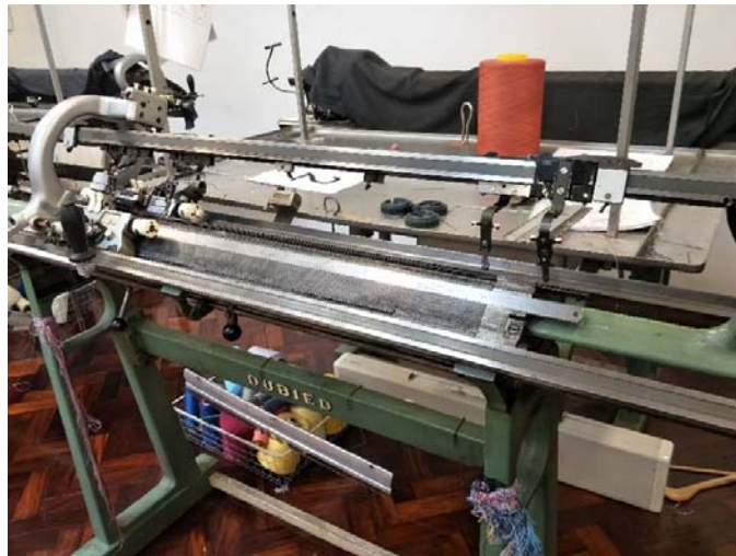
Figure 3.18 Double-bed flat knitting machine (10-gauge).
