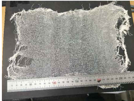
Figure 7.3 PP-40 circular plain jersey knitted fabric after treated with toluene.
