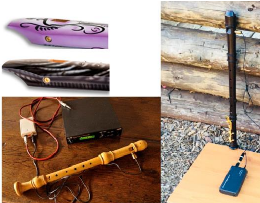
Figure 19 (top-left). ‘Elody’ designs (two examples of many) by Mollenhauer Company: heads with integrated pick-up. 89
