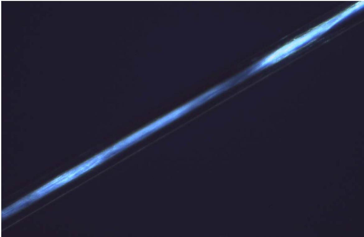
Figure 30: Silk birefringence. The proteins start to align and show birefringence when flown through a glass capillary only at very high speeds.
