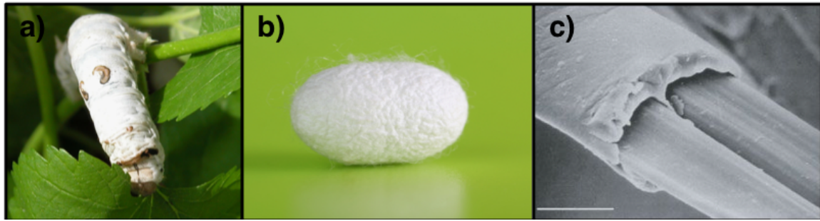
Figure 3: Bombyx mori silkworm silk. a The Chinese silkworm Bombyx mori . b Cocoon spun by the silkworm Bombyx mori . c Structure of the Bombyx mori silk fibre. The two fibroin monofilaments are covered by a sericin layer. Scalebar: 10 \mu\text{m} . Reprinted by permission from Springer Nature: Nature, Surprising Strength of Silkworm Silk, Shao and Vollrath), Copyright 2002.
