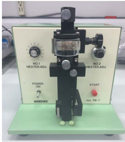
Figure 24: Narishige PB-7 glass capillary puller.
