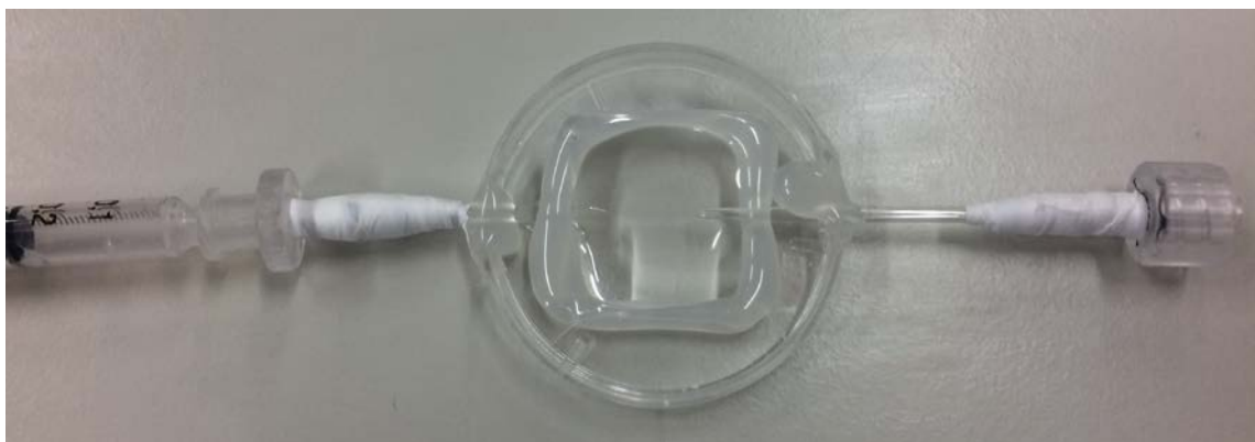
Figure 28: Silk flow visualisation setup 2. A glass capillary with a tapered middle part was accessed at both ends to push and suck the proteins through the duct. A glass cover slip is glued to a petri dish with hot melt glue to allow visualisation under polarized light.
