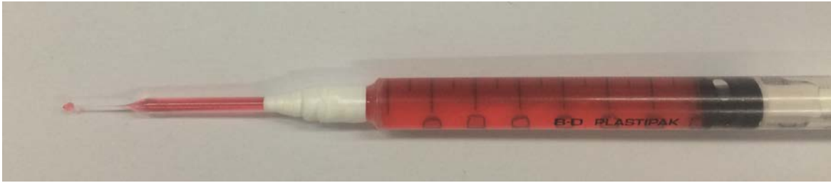
Figure 27: Silk flow visualisation setup 1. Pushing a glass capillary into the opening of a 1 ml syringe and fixing it with PTFE tape to prevent it from leaking. The syringe in this picture is filled with a red food colour/water mixture for better visualisation.
