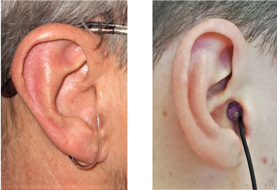
(A) Probe microphone at the eardrum with an open ear canal, reproduced from Griesinger (2013) (B) Microphone at the entrance to a blocked ear canal, reproduced from Armstrong et al. (2018a)
