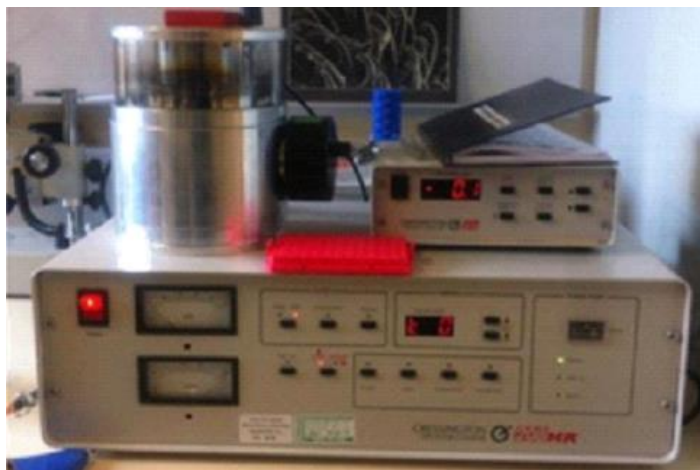
Figure 2.5 Sputter Coater used to coat sample with platinum.
