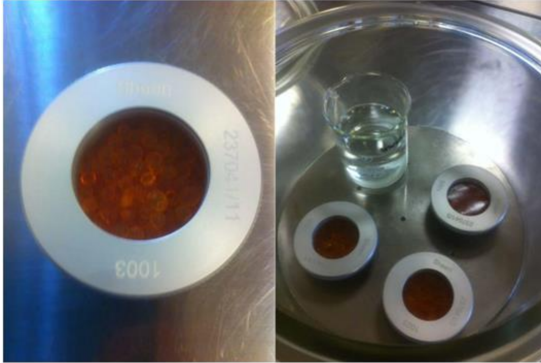
Figure 2.6 Picture of permeability cup (Sheen UK), (b) Permeability cups with saturated salt solution in desiccator.
