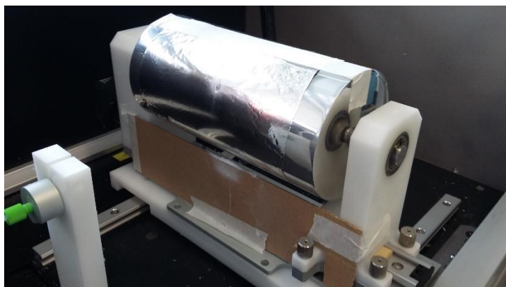
Figure 6.6.2 A: Cardboard wind-breaker for spinning aligned scaffolds. On the Bioinicia rig.
