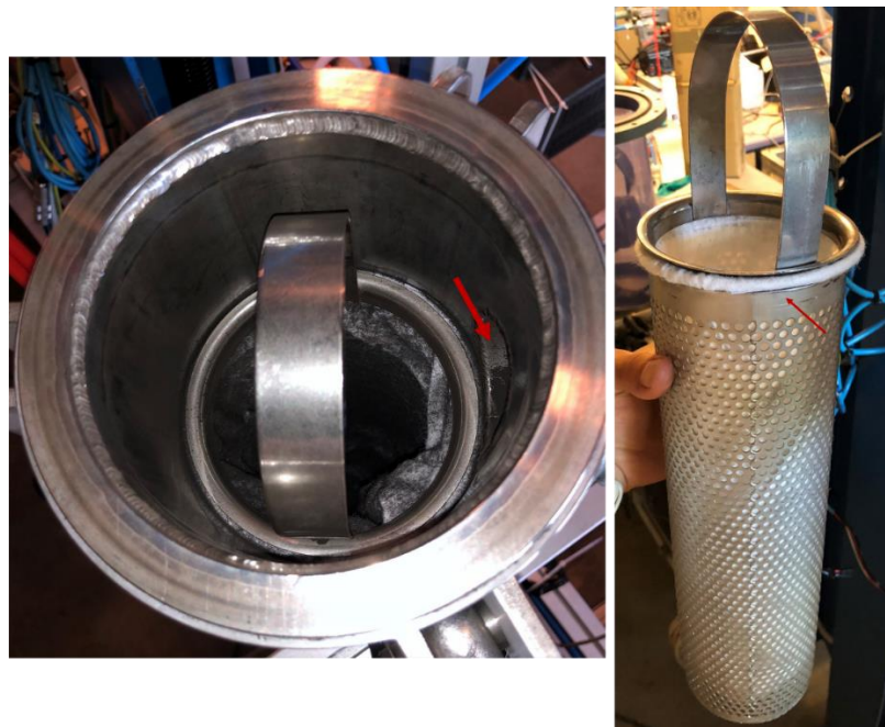
Figure 5-13. Respectively on the left and right: stagnant fines at the entrance of the filter housing and leaking perimeter of the sleeve filter
