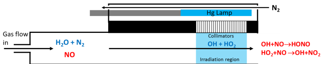
Figure 3.10. Calibration wand showing the reactions used to generate HONO.
