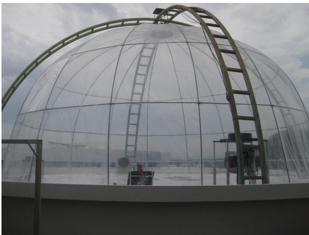
Figure 5.3. The chamber used in the experiments described in this chapter. The inlet for the FAGE cell, not visible, was located on the opposite side of the chamber.
