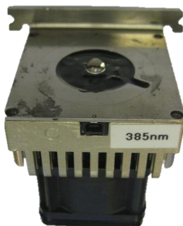
Figure 3.13. LED used initially to photolyse HONO. The lens is visible in the centre with the LED mounted beneath.
