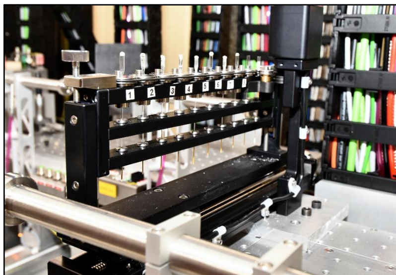
Figure 3.6. Long-duration experiment (LDE) sample stage set-up. Numbers indicate the different cement samples being analysed.
