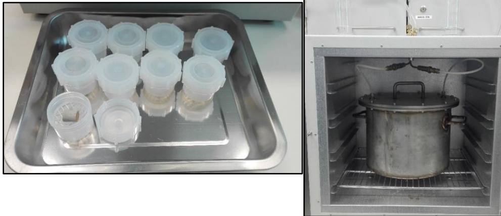
Figure 3.1. (a) Cylindrical monolith placed inside a 60 mL Teflon vessels; (b) Stainless steel “bean tin” being purged continuously with nitrogen gas.
