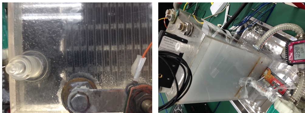
(a) floating undissolved zinc deposition after discharging phase
