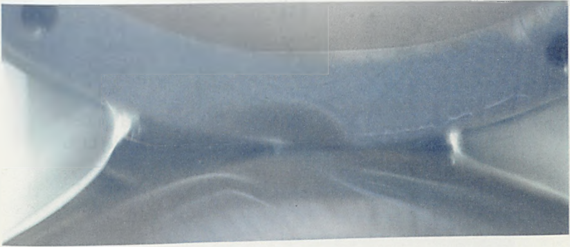
Figure 1.3: An Experimentally-Obtained View of the Nip Region of a Fully-Flooded Forward Roll Coater (Malone [1992])
