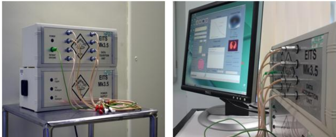
Figure 2.5: The Sheffield Mk 3.5 aEIT system.
