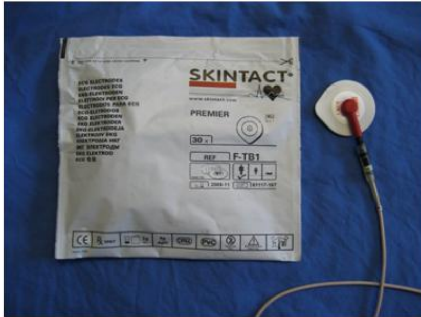
Figure 3.2: Skin surface electrodes used for aEIT system.
