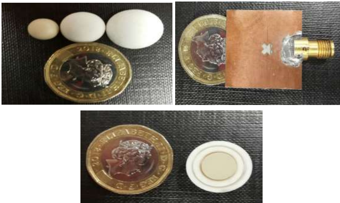
Figure 5.17: Prototype of a multi-layer mm-wave hemispherical DRA before and after assembly.
