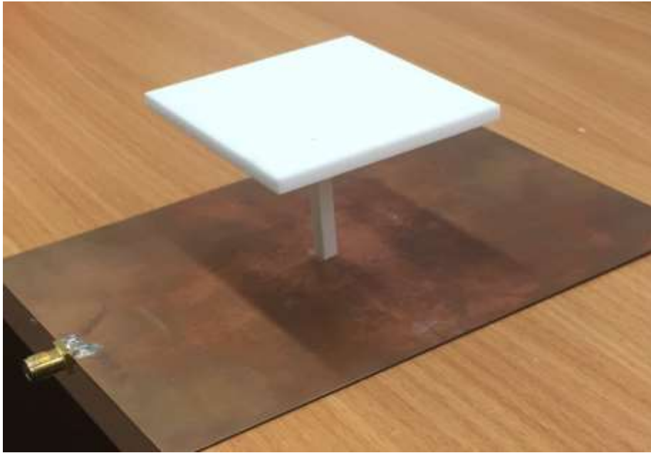
Figure 2.26: Dielectric superstrate overhead rectangular DRA.
