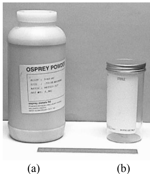
Figure 2.1: (a) Powder storage container, as supplied and (b) spent and mixed powder storage. A 6inch rule is pictured.
