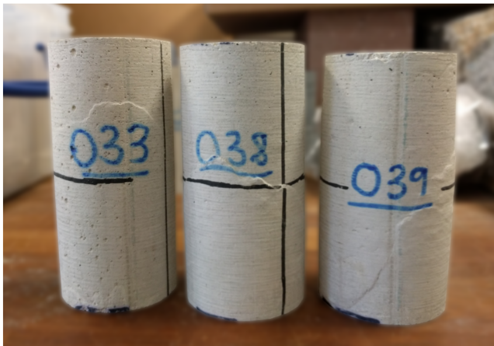
Figure 4.13: Three specimens of Ordinary Portland cement composition (Table 4.2) after testing under triaxial conditions. Specimen #033 at 5 MPa \sigma_3 . Specimen #038 at 10 MPa \sigma_3 . Specimen #039 at 15 MPa \sigma_3 .
