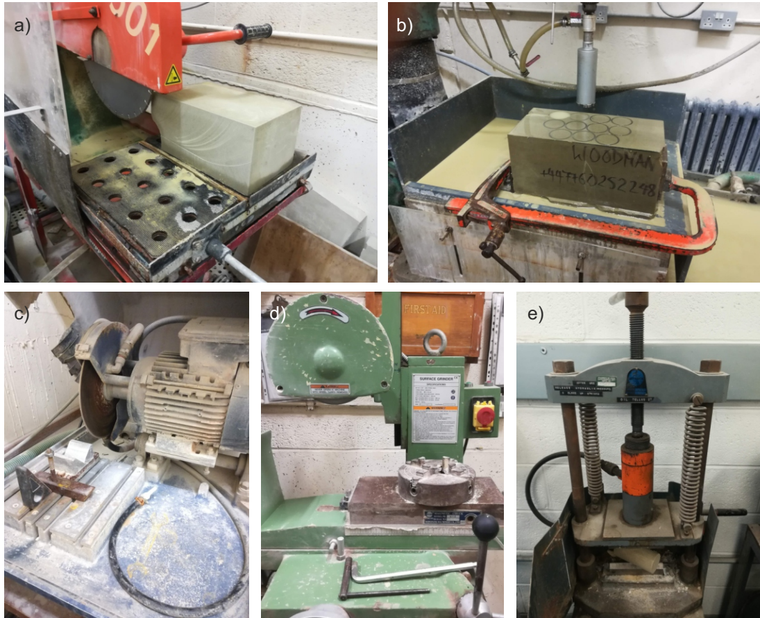
Figure 3.1: a) Sawing dimension stone blocks to maximum dimensions of 40 x 40 x 20 cm with diamond sintered circular saw. b) Coring cylindrical specimens at 54 mm diameter with diamond impregnated drill bit. c) Trimming specimen lengths to \approx 120 mm using a diamond sintered circular saw. d) diamond sintered grinding wheel for grinding specimen ends. e) Inducing discontinuities in specimens at an angle of 30^\circ to 40^\circ by tensile splitting.
