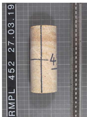
Figure B.3: Photographs of intact specimens of Midgley Grit after thermo-mechanical triaxial testing.
