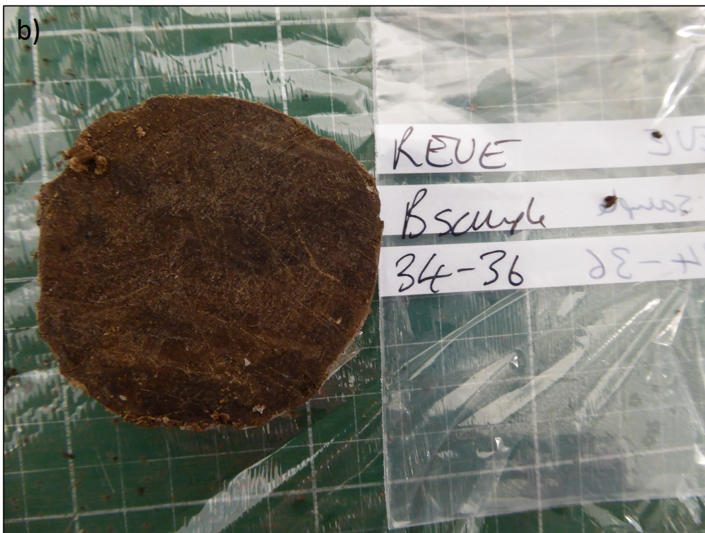
Figure 2.5 Photographs showing a) coring the active layer and shallow permafrost of Adventdalen in spring 2016, using body weight to force the drill down (Credit: Ebbe Bak), and b) a slice of core R1b from a depth interval of 34-36 cm. The squares on the green cutting board are 1 cm 2 .
