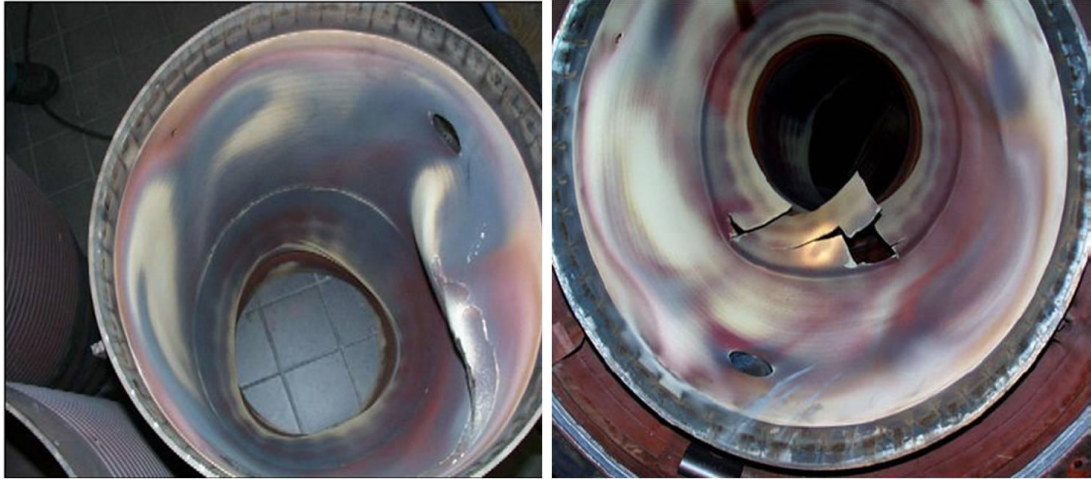
Figure 1.1: The damaged combustors due to the thermoacoustic instability. [5, 6]
