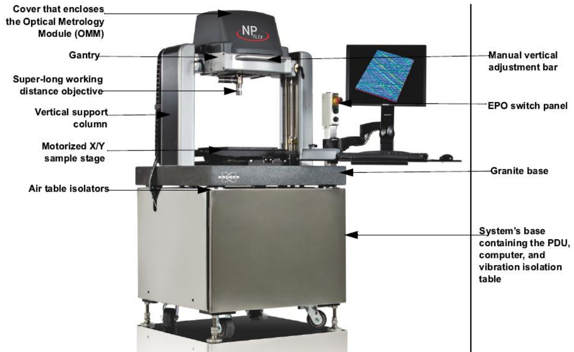
Figure 3-14: Image of the Bruker NPFLEX Interferometer system.
