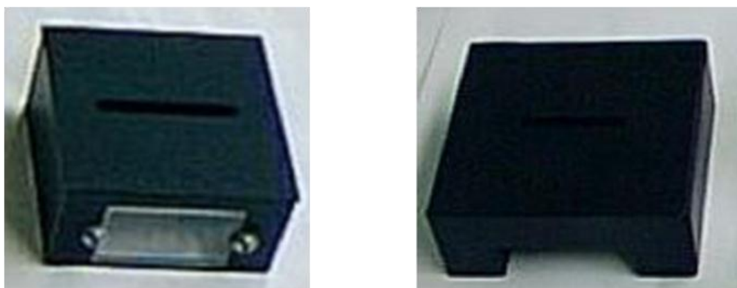
Figure 3-2: Picture of the ceramic chamber, constituted of two borosilicate glass viewing windows embedded in the side-walls, used to protect the experiment from the atmospheric contaminants and to measure the surface tensions and apparent contact angle \theta_{ACA} of the different systems.
