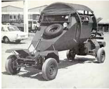
Figure 1.10: A Leopard infantry carrier used in the Rhodesian bush war. The heavily V-shaped hull is displayed, alongside other defensive adaptations to landmine blast. Taken from the work of Ramasamy et al [14]
