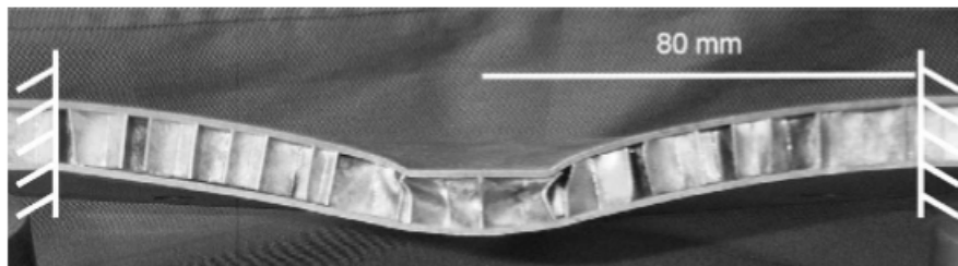
Figure 1.15: Deformation of a real square-honeycomb structure of the type shown in Figure 1.14. Taken from the work of McShane, Radford, Deshpande and Fleck [55]
