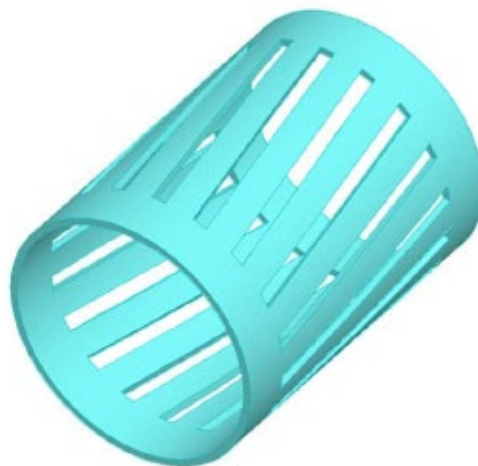
Fig.1.30. Sleeve grooving for eddy current loss reduction [SHE13].
