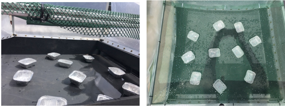
Figure 3. 7: ( Left ) Containers were randomly placed on the test bed; ( Right ) Water applied from rainfall simulator frame height, through a diffraction mesh to test spatial distribution of water.
