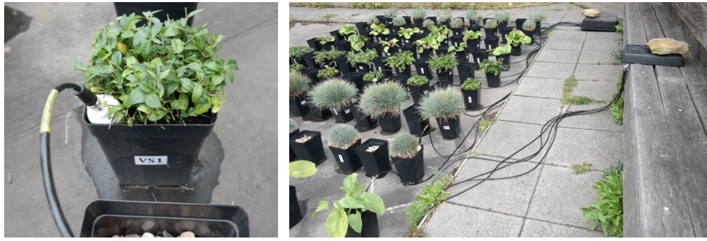
Figure 2. 6: ( Left ) SM150T moisture sensors were installed in the soil of one plant sample of each species; ( Right ) Moisture sensors were connected to GP data loggers.
