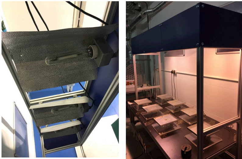
Figure 2. 9: ( Left ) Three sodium lights for artificial daylight effect; ( Right ) The effect of the lightings above the load cells.
