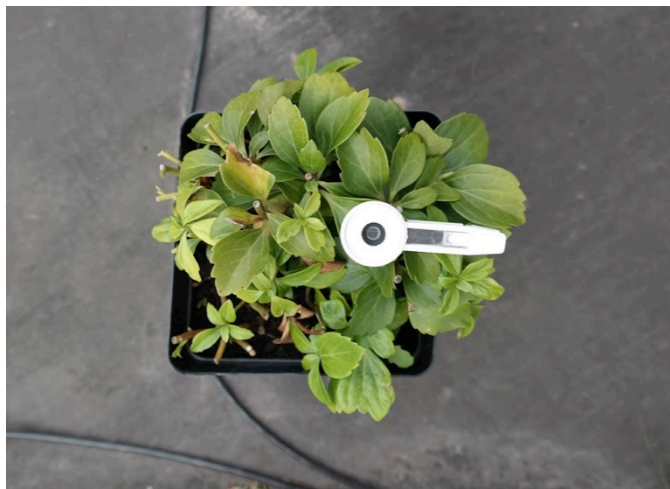
Figure 2. 7: Leaf clip attached to random leaf sample with the shutter closed for darkness adaptation to measure chlorophyll fluorescence.
