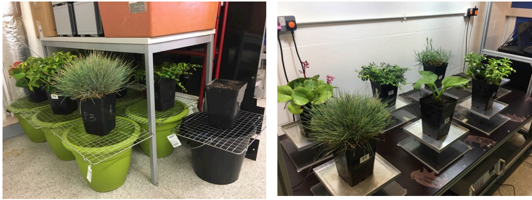
Figure 5. 1: ( Left ) Treatments drained for 2 hours to reach field capacity after being submerged for 20 hours; ( Right ) Treatments placed on load cells for continuous weight change monitoring.
