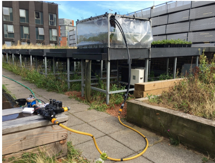
Figure 2. 4: Rainfall simulator attached on the test bed and connected to valve for water supply.
