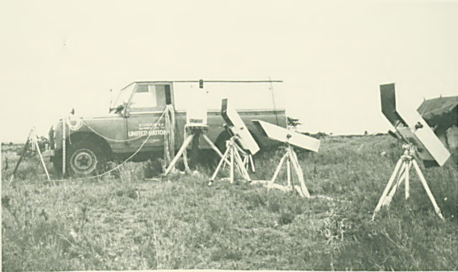
PLATE 2 Mark I receivers with weather shrouds fitted. The Mark II (two-channel) receiver can be seen next to the Landrover.
