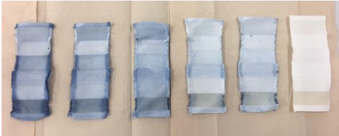
Figure 3.31: Multifibre after washing with denim in water at altered pH. From left to right: pH 3, pH 5, pH 7, pH 9, and pH 10.6, unwashed multifibre.
