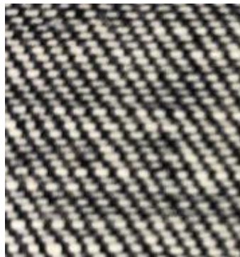
Figure 3.1: Close up picture of the back of denim material showing indigo dyed cotton warp and white cotton weft.
