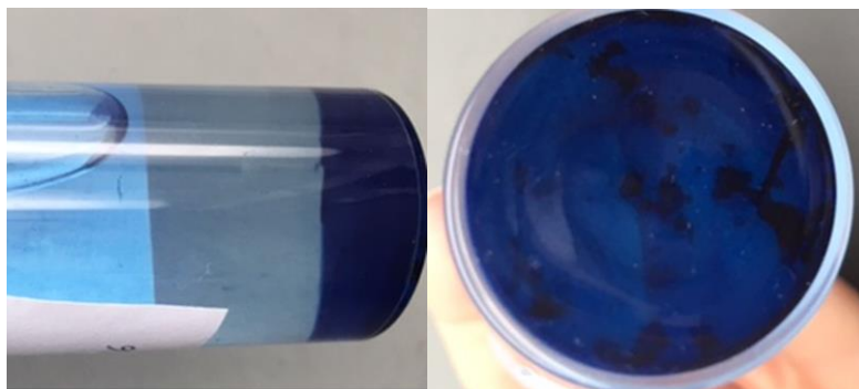
Figure 3.13: Images of filtered denim wash liquor in distilled water after 5 months. A blue solution can be seen (left) but blue precipitates have also formed at bottom of sample vial (right).
