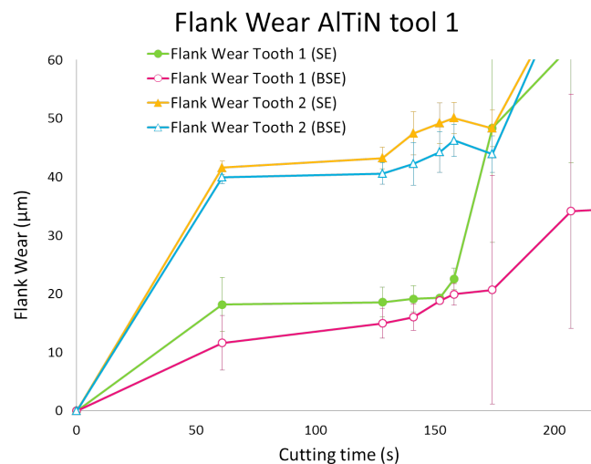
Figure 9.12: Although there is suggestion of a wear curve in the raw data, the averaged data is not conclusive due to high uncertainty.
