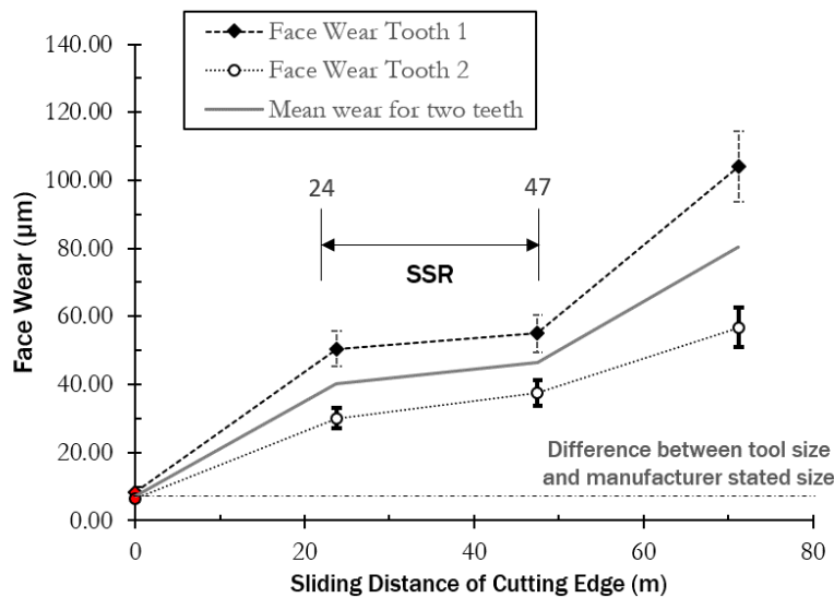
Figure 5.12: Tool wear curve measured for face wear of tool used to machine Hastelloy C-276. Red points indicate how much smaller new tool is compared to manufacturer stated size 500 \mu\text{m} . Starting size is shown with dotted line.
