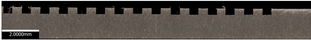
Figure 5.6: Image of the workpiece sectioned perpendicular to direction of cut. Cross section of the slots machined can be seen.
