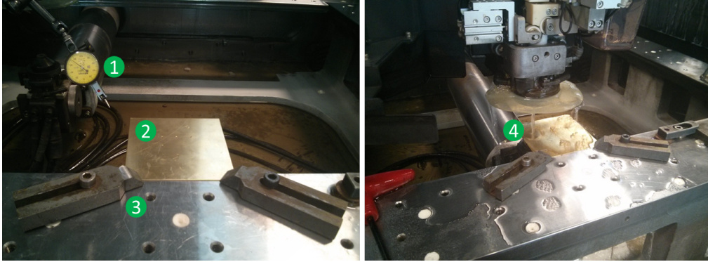
Figure 3.2: Clamping system for workpieces. | 1. Dial gauge for squaring workpiece | 2. Pre-drilled workpiece | 3. Clamps | 4. Water jet for threading |
