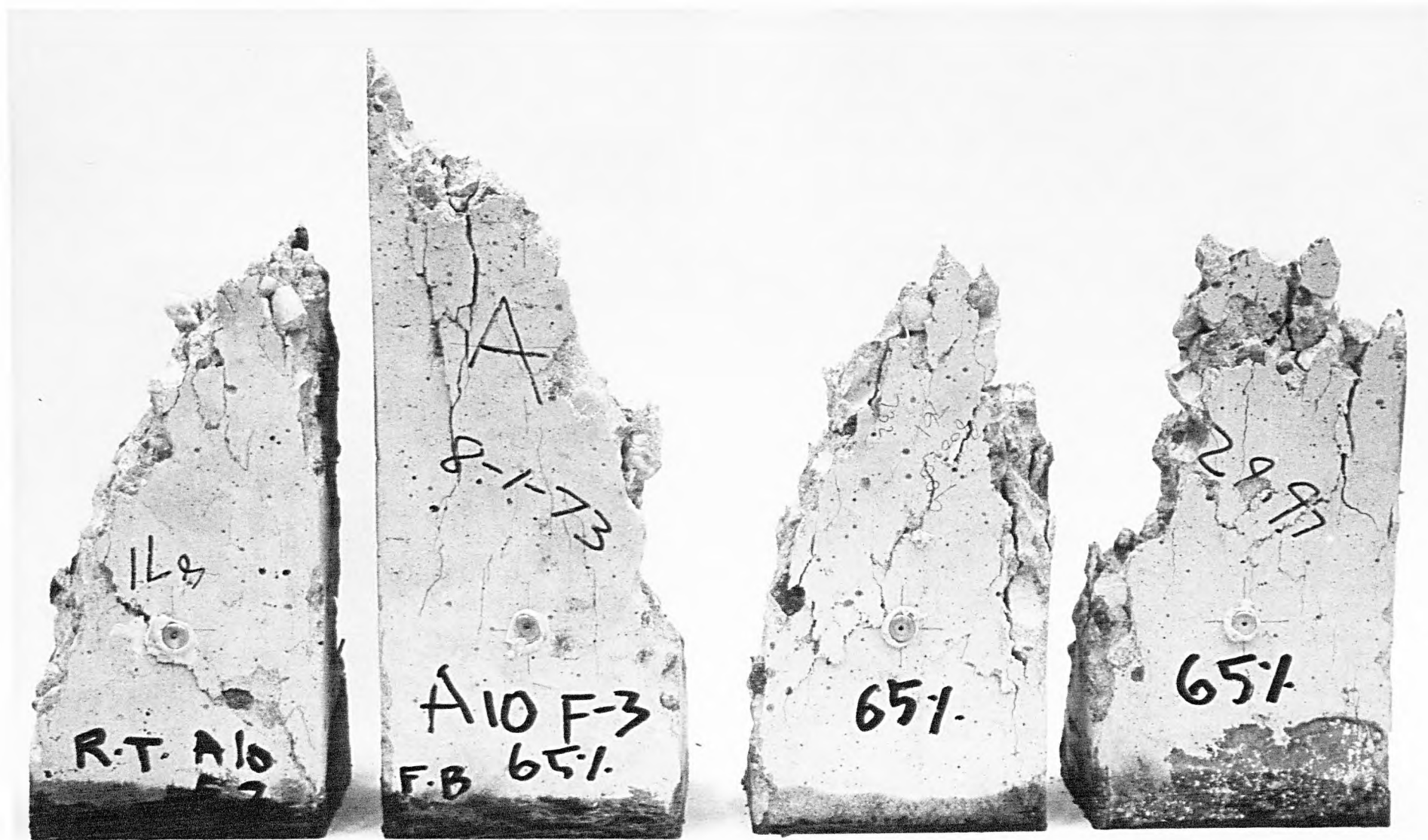
PLATE 5. FATIGUE FRACTURE MADE IN LOW STRESSED SPECIMENS.
