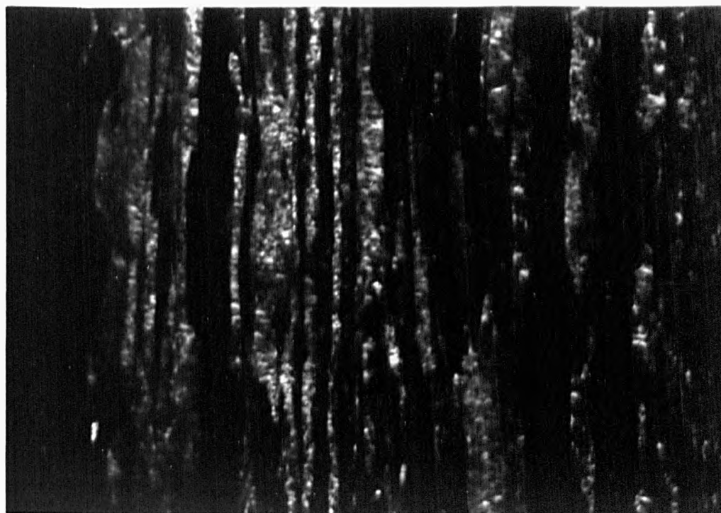
Figures 3-5. TEM (002) dark-field images from longitudinal sections of MP-based carbon fibres : E35C, E35, E55, E75, E105, E120, E130, and C700)
