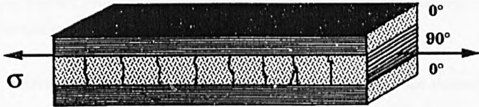
Fig. 1.3 A symmetric [0^\circ/90^\circ/0^\circ] laminate with transverse cracks in 90^\circ ply
